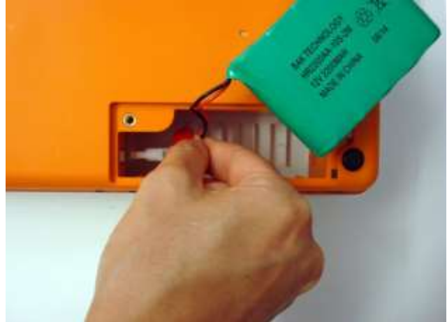
2. Disconnect the battery connector.
