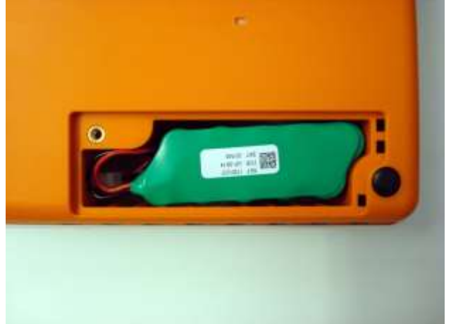
4. Place the battery in its compartment.
